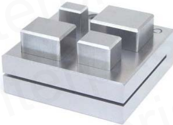
DSC-033 4pc Square and Rectangle Disc Cutter Set Cut Sizes: Square: 10mm, 15mm, 20mm Rectangle: 15mm x 25mm Material Steel Available in Wooden Box Available with Allen Key Tool or Locking Lever
