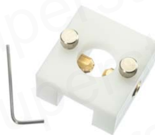
BDT-023 Bead/Pearl Holding Vise 2 Brass Cupped Jaws to hold bead Dimensions: 2" x 2" x 1" Hole Diameter : 21.3mm Hole Accepts approx 1mm drill Drilling from both sides
