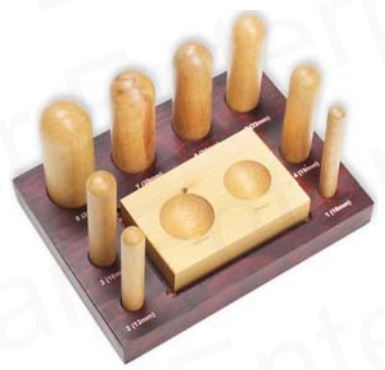
DBP-515 10pc Wood Dapping Block & Punch Set 8 Punches 10 - 31mm (3mm increments) Holes: 11 - 32mm
