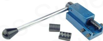
RER-005 Ring Bender Ring Bender 2 Forming Dies: -Half Round -Flat
